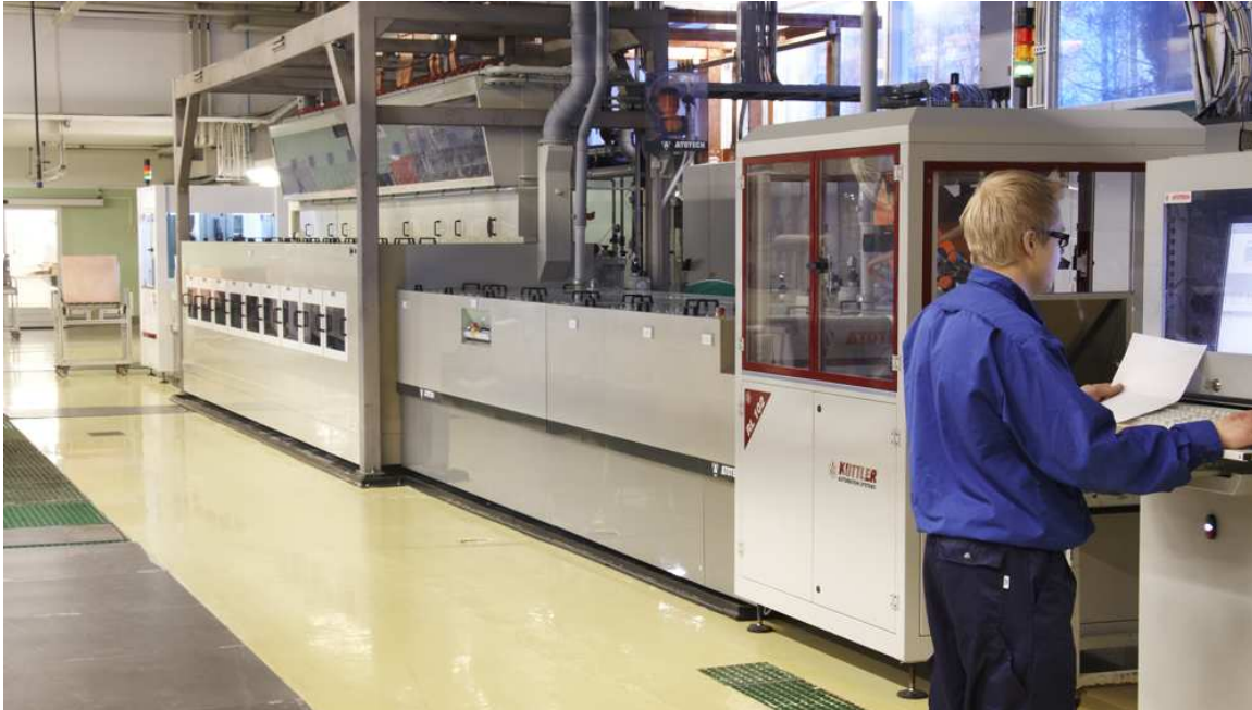
Pic 4. A large machine to make small PCBs. Copper plating line in Oulu.
